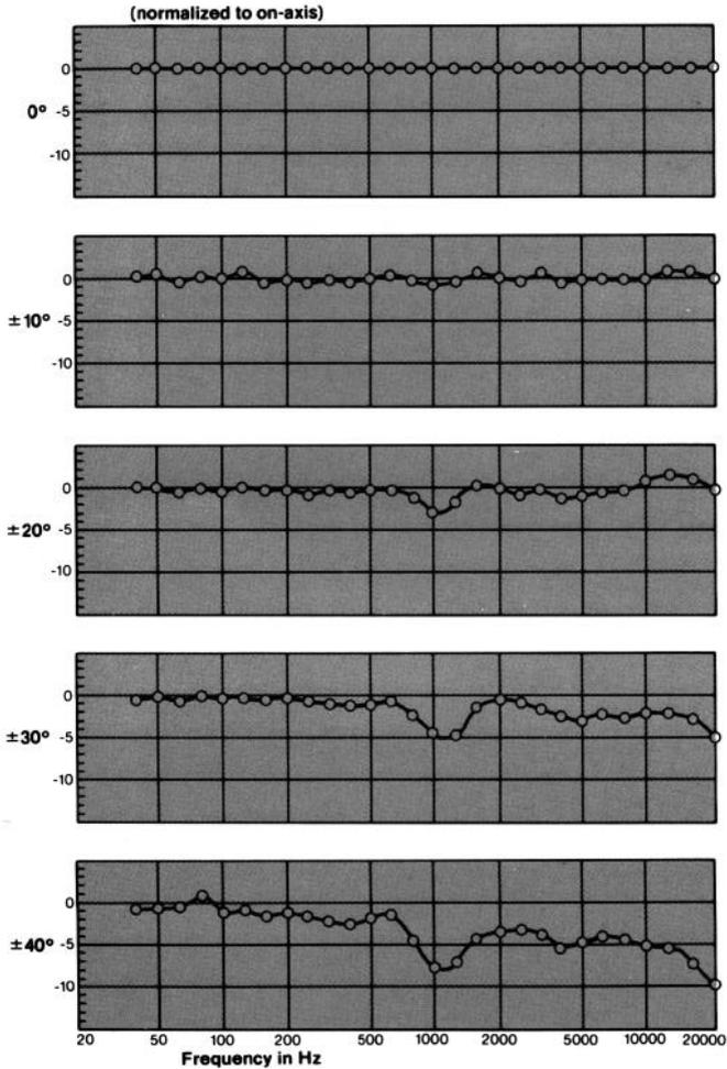
Figure 5. Vertical Off-axis Response (normalize to on-axis)
