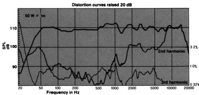
**Figure 16. Distortion vs. Frequency (4435)**
