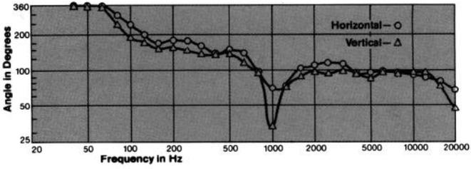
Figure 3. Directivity vs. Frequency (4430)
