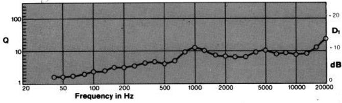
Figure 4. Horizontal Off-axis Response
