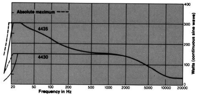
Figure 12. Maximum Continuous Output
